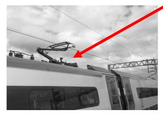
Electrical voltage + current (+ spikes) Vertical forces (time-varying) Longitudinal forces due to friction Heat Flash arcing Electromagnetic field flux (+RFI) Vibrational forces (resonance?) Shock (at joints)
