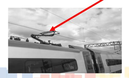
Electrical voltage + current (+ spikes) Vertical forces (time-varying) Longitudinal forces due to friction Heat Flash arcing Electromagnetic field flux (+RFI) Vibrational forces (resonance?) Shock (at joints) Moisture & salt deposition Carbon deposits, rust, crud
