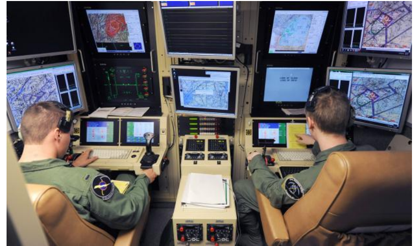
Predator Unmanned Aerial System Cockpit (Photo: www.mitre.org )
